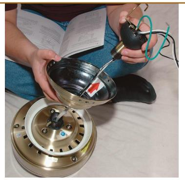
Save yourself a headache. Once you've identified all the parts, thread the wires through as you assemble the fan motor, canopy trim ring, canopy, and base. Make sure the parts are assembled in the right order now, rather than later. Don't attach the blades until the fan body is in place.
