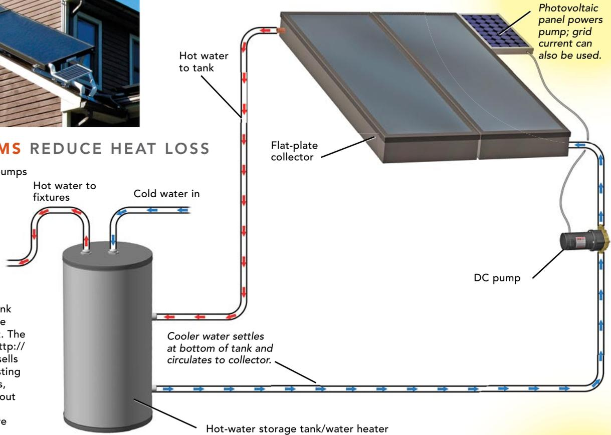
Photovoltaic panel powers pump; grid current can also be used.
