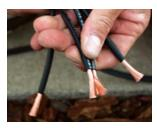
3. Keep the polarity of the cable consistent: One of the wires will have longitudinal ribs. Keep them together.
