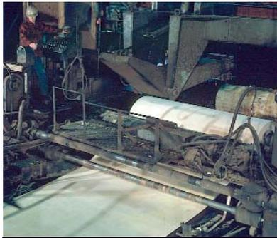
**Grain orientation provides strength.** Peels from a log are laid up by alternating the grain direction of each ply at 90° to the one below it.
