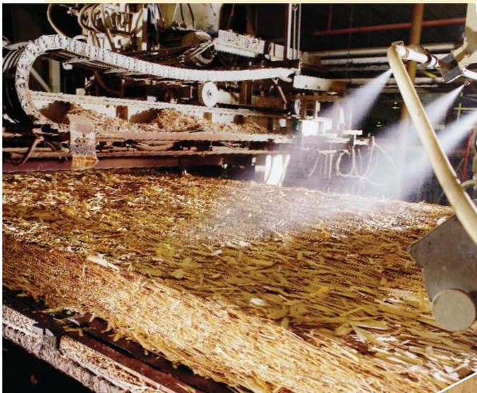
**Strength in numbers.** Each layer of thin, narrow wax-and-resin-coated wood strands is arranged with its grain direction oriented 90° to the layer below, just like plywood. The cross-lamination of thousands of strands provides strength in both directions without knots or voids in the panel. Spray nozzles maintain proper moisture content until the mat reaches the press.
