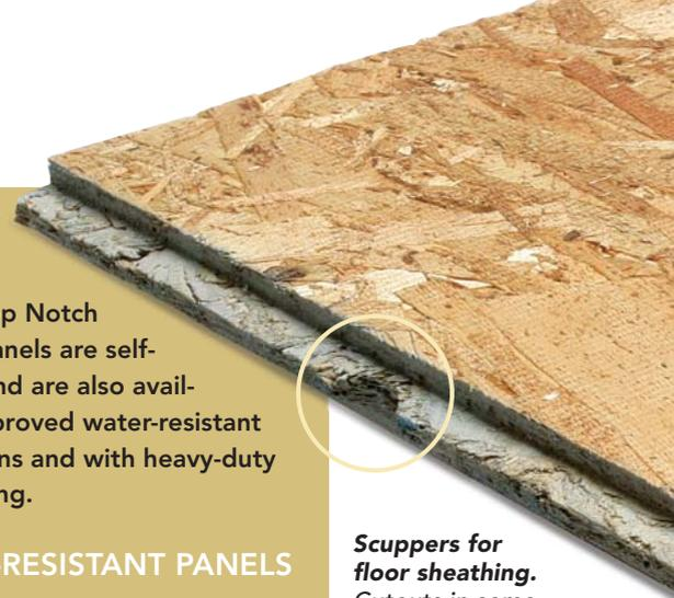
**Scuppers for floor sheathing.** Cutouts in some brands of Louisiana-Pacific's tongue-and-groove floor sheathing drain water. Notches on the underside of the 4-ft. ends also prevent water from pooling on the joists.
