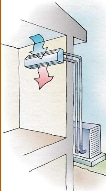
For example, the Mitsubishi Mr. Slim Hyper-Heat unit (model PUZ-HA36NHA) has a nominal heat-output rating of 38,000 Btu/hour. According to the manufacturer, at an outdoor temperature of  $-13^{\circ}\text{F}$ , its heat output drops 21%, to 30,000 Btu/hour. If your heating-design temperature is  $-13^{\circ}\text{F}$ , you would assign the unit an output rating of 30,000 Btu/hour, not 38,000 Btu/hour.
