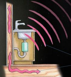
Noise travels through a house in two ways: through the air and through solid structures. Airborne sound can be absorbed by porous materials like fiberglass insulation, and structure-borne sound can be stopped by heavy, dense materials like the mass-loaded vinyl being installed in the photo at left.
