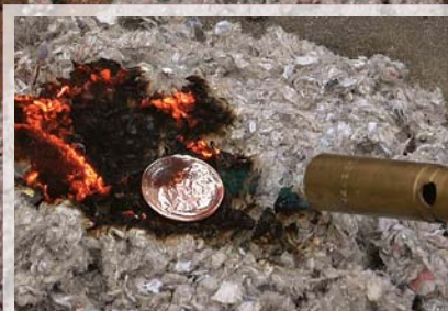
Penny wane. A propane torch will melt a penny but won't burn cellulose insulation.
