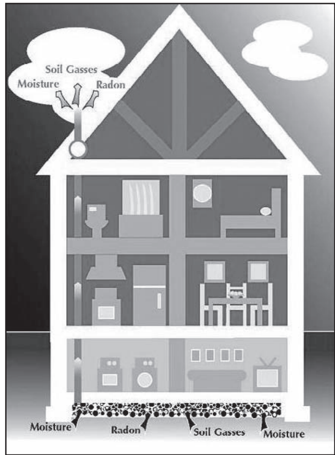
Figure 2. HomeAire advertises that its radon mitigation systems help dry out damp basements.
